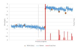
Figure 2: Partway through a bioreactor MSC expansion process, the glucose is adjusted from 2g/L to 4g/L, which is automatically performed via Smart Perfusion. As the cells consume glucose, a pump automatically feeds in fresh glucose to maintain the set point (red peaks).
